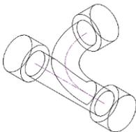
**NOTE** The size of this component is 4" (100mm). It is a typical PVC swept tee for plumbing purposes.
