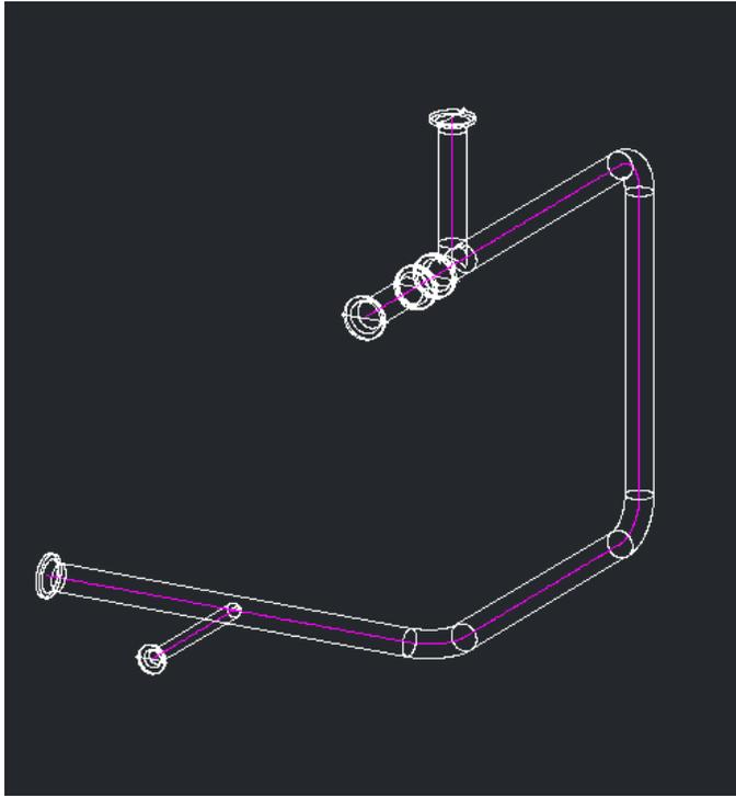
2. Click **Plant > Accessory > CAESAR II > System Out**. Alternatively, type **C2OUT** on the command line and then press ENTER.
