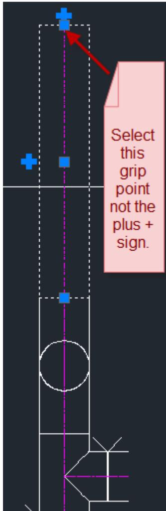
10. Drag the pipe down to the top of the pipe rack so that it is on the same line.
