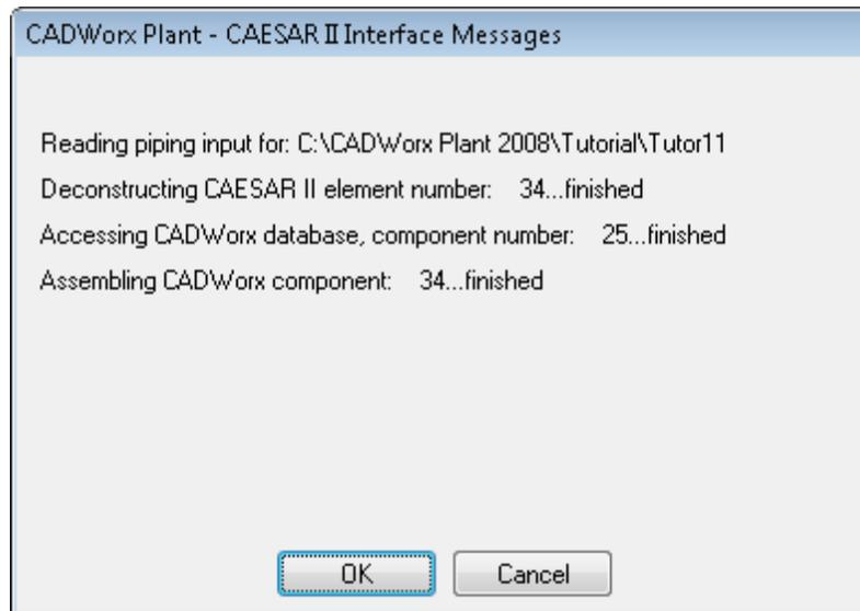
*After reading the input file, the next prompt requests the level of intervention required. For more information, see "System In" in the CADWorx Plant User's Guide.*
