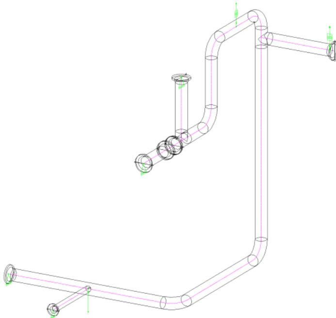
29. Click **Plant > Accessory > CAESAR II > System Out**. Alternatively, type **C2OUT** on the command line, and then press ENTER.
