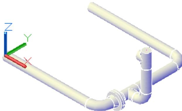
When you insert a reducing component--such as the concentric reducer--the main size and the reduction size default large to small providing the proper connection at the reducer. After inserting a reducing component the main size and the reduction size reverse. This allows placement of other components on the pipe run without having to reset the sizes.
