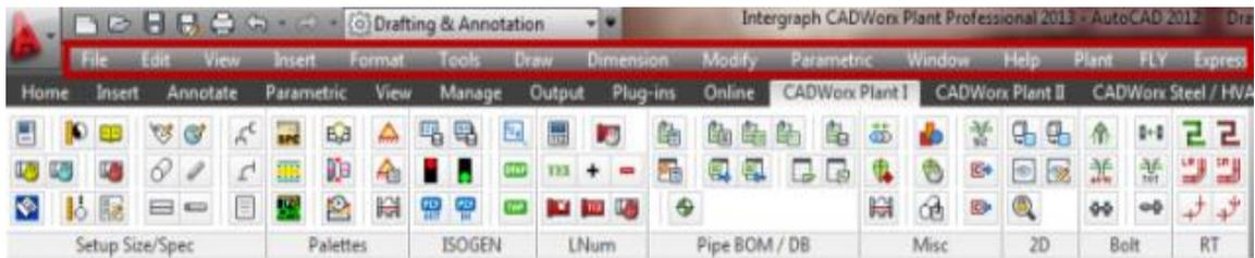
The quickest way to access CADWorx Plant toolbars is to click **Plant > Toolbars**, and then select a toolbar in the list. The toolbars displays in the drawing environment, where it remains until it is removed.
