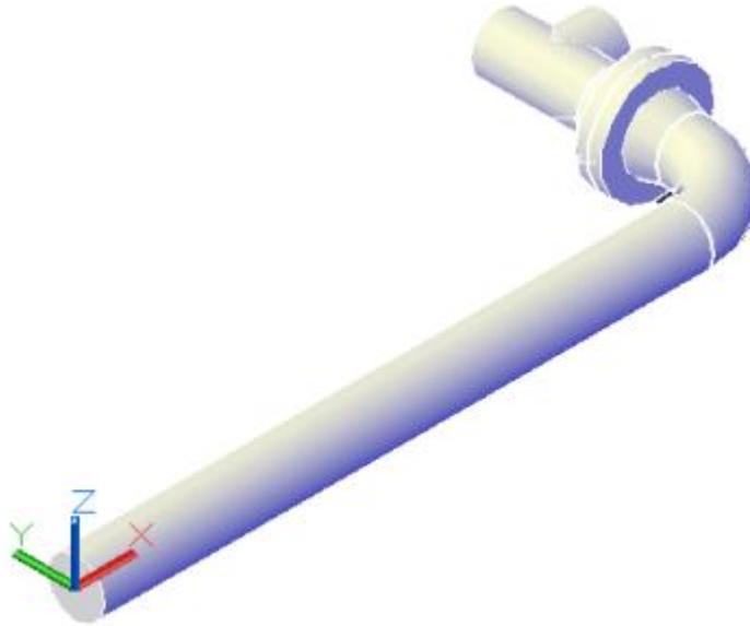
*The tee is placed, and the program places you back at the north point of the model on the other end of the tee.*
